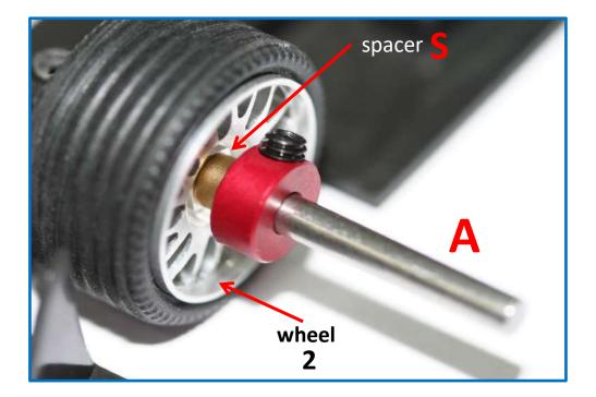
At the other end of the axle **-A-** you must place the 1 or 2 mm spacer. -just touching the rim- and the stopper -also touching the spacer- as can be seen in the upper picture and in the lower drawing.
