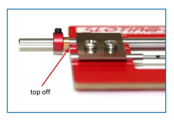
Position the axle -B- (touching the axle -A-) and finally fix the stopper -C-. The measurement reflected in axle -B- will serve as a base to finally create the -RIGID AXLE FOR INDEPENDENT WHEELS-.
