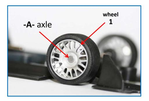
VERY IMPORTANT: Assemble one end of the front axle **-A-** as indicated in the picture above, taking special care to make the axle at level with the rim. It's not important the model or type, the most important thing is that the rim is perfectly at level with the axle as indicated in the lower drawing.
