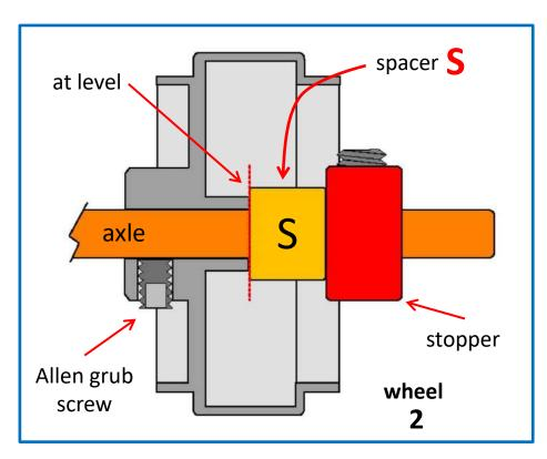
ATTENTION: Remember to always leave a little lateral clearance between 0.20 and 0.40 mm. so that the wheels can turn freely.
