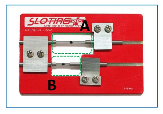
In order for the axle we are manufacturing to be perfectly straight, it is very important that the right side semi-axle it's not "hanging up" and be well supported in the groove.
