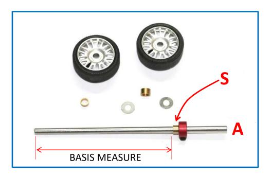
Then you can place the axle **-A-** as indicated in the photo below, just a "top off" with the red base.
