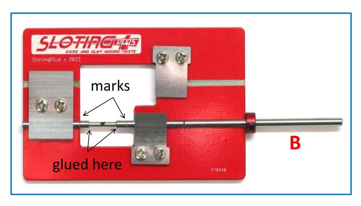
ATTENTION: Glue the set with Cyanoclirate type glue but using **-VERY LITTLE AMOUNT-** quantity because the glue will act by capillarity and a very small quantity is sufficient. Help yourself with a toothpick or similar to deposit the glue.
