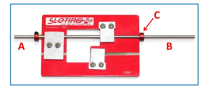
Now place the two semi-axles, taking special care that the marks are facing each other (lower image) and also place the small guide axle inside.
